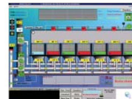
Operation of the post-combustion unit showing the monitoring of inlet and outlet chambers, the fans operation with data on flow rate, temperatures and pressures as well as the burners' performance.
