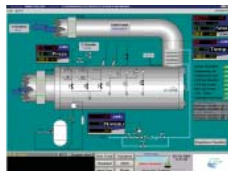
Diagram of the recovery boiler. The chart below shows data on flow rate, pressure, steam generation and outlet temperatures.
